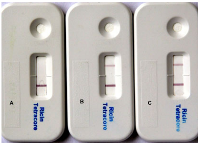
FIG. 6—Detection of ricin on immuno-chromatographic strip after denaturing ricin in boiling water for various time intervals. A: Control; B: 15.0 min boiled; C: native ricin; ricin.
