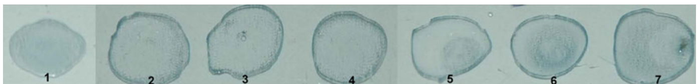
FIG. 4—Detection of ricin by Latex agglutination test after denaturing ricin in boiling water at various time intervals. 1: Control; 2: ricin; 3: 3.75 min boiled ricin; 4: 7.5 min boiled ricin; 5: 15.0 min boiled ricin; 6: 30.0 min boiled ricin; 7: 60.0 min boiled ricin.
